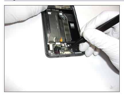
After removing the band, gently lift the audio jack out of the phone.
