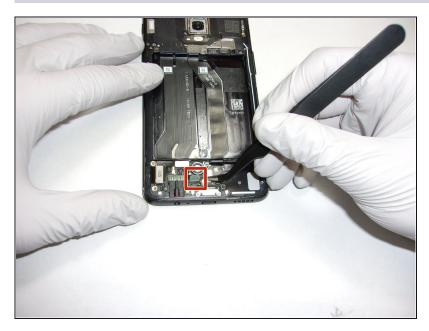
Use tweezers to gently pull away the tab securing the audio jack to the speaker assembly.
