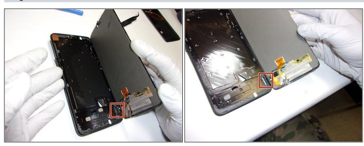
• After gently prying the screen from the frame, carefully thread the tab through the bracket to remove the screen from the phone.
