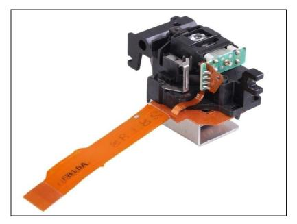
• Once the laser lens is carefully separated from the optical drive assembly, insert the new laser into the optical drive assembly and follow these steps in reverse order for reassembly. To reassemble your device, follow these instructions in reverse order.
