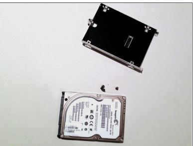
To remove the hard drive from the bracket remove the two M3.0×4.0 screws from each side of the hard drive.
