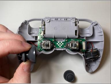
Grab the top and pull straight up on the joystick cap. Pulling out the caps one-by-one.
