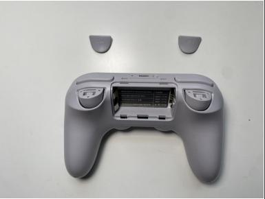
Remove L2 and R2 trigger buttons by pushing them away from the grips.
