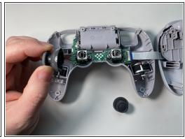
Grab the top and pull straight up on the joystick cap. Pulling out the caps one-by-one.
