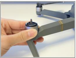
Pull up the propeller to remove it.
