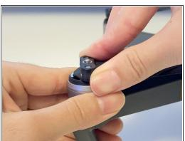
Push down slightly on the propeller you want to remove.
