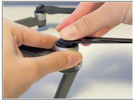
If the propeller you want to remove DOES NOT have a white outline, then turn the propeller clockwise to unlock its position.
