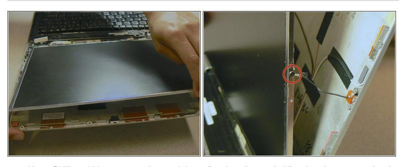
Use a Phillips #000 to unscrew the one 2.8 mm fine thread screw holding the wire connected to the right face of the LCD.
