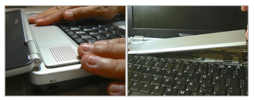
Remove the rest of the cover by sliding it to the right and lifting the right edge.
