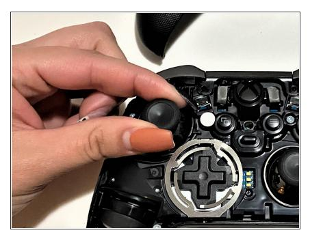
Replace the analog stick, and twist to the right until it tightens.
