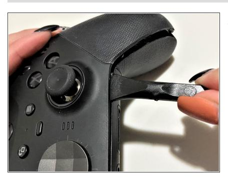
Slide the prying tool along the crease of the bottom of the controller.
