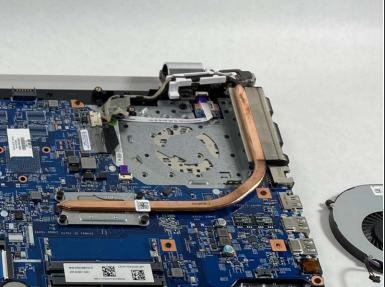
Remove the fan from the device.
