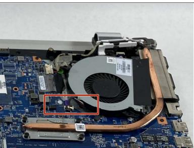
Disconnect the fan wire carefully so that the fan is longer connected to the motherboard.
