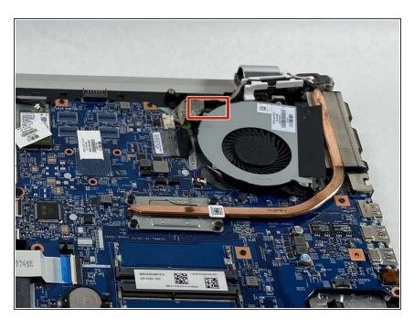
Use a Phillips #0 screwdriver to remove the single screw securing the fan to the motherboard.
