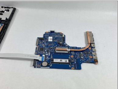
Gently lift and remove the motherboard from the device.
