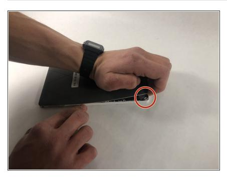
Peel the back cover off of the Kobo Arc by finding the lip in the cover and pulling back on it.
