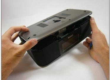
⚠ The bottom cover is attached to the back cover by two plastic clips. Don't use excessive force.
