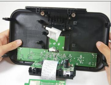
• Use a plastic opening tool to pry and lift up the white zip connector holding the LCD screen to the buttons.
