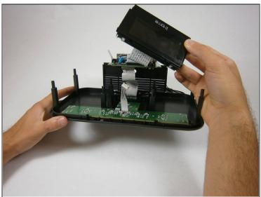
Gently push the screen away from you to dislodge it from the plastic clip holding it in place and then pull up to remove.
