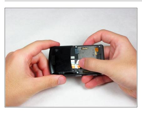
Remove the SIM card by pulling it toward the top of the phone with your thumb.
