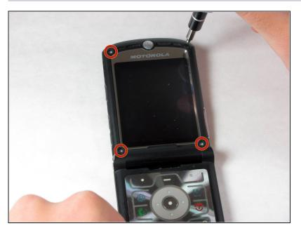
Remove the four T5 Torx screws that were underneath the rubber covers.
