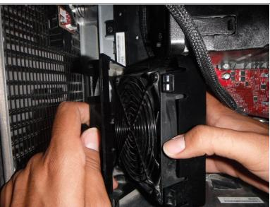
Disconnect the fan from the cage housing by pressing down on the release triggers and pushing them to the right.
