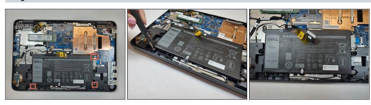
Use a Phillips #0 screwdriver to remove the three 3 mm screws from the battery.
