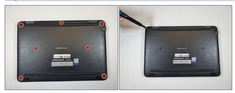
• Use a Phillips #0 screwdriver to remove the seven 7 mm screws securing the back case.
