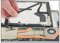
• Pry up with the flat end of a spudger to disconnect each display cable from the motherboard.
