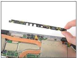
• Carefully remove the antenna support bracket.
