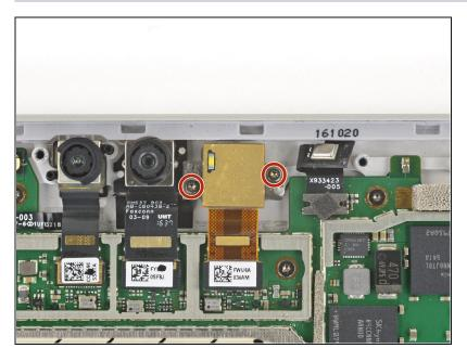
Use a T3 Torx screwdriver to remove the two 2.2 mm screws securing the rear camera.
