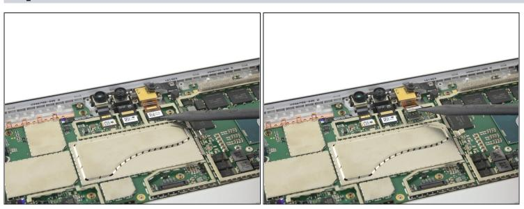
• Use the pointed end of a spudger to disconnect the rear camera from the motherboard.
