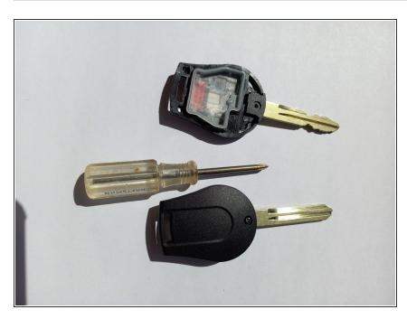
Place the cap back on the new key and screw everything back into place. Test the key on your vehicle to make sure that all the buttons work.
