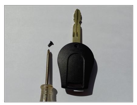
Using the Phillips #0 screwdriver, remove the single screw securing the key fob shell.
