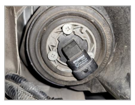
Align notches and insert the headlight bulb into the socket.
