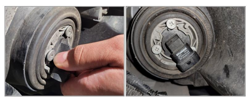
Turn the headlight counter clockwise to release it from the headlight assembly.
