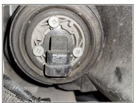
Remove the headlight connector by depressing the clip and pulling it away from the vehicle.
