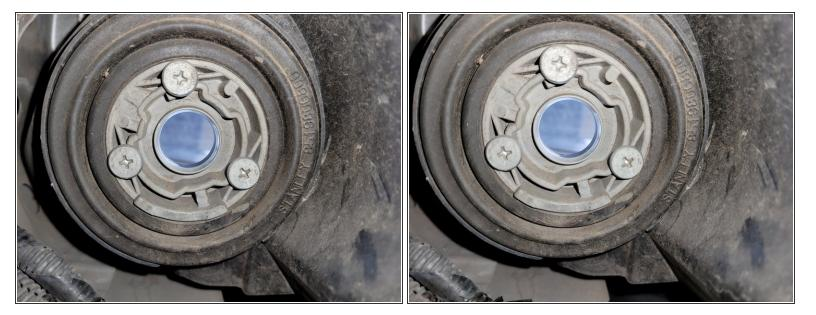
Pull the headlight bulb out of the socket.
