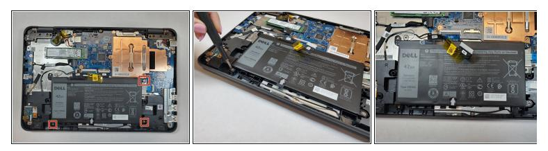
• Use a Phillips #0 screwdriver to remove the three 3 mm screws from the battery.
