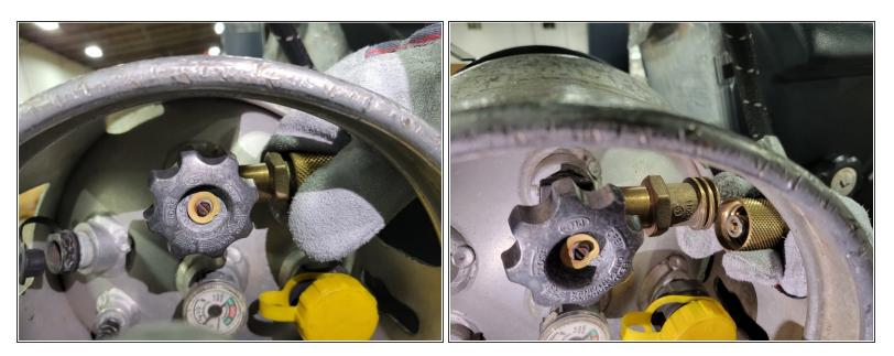
• Disconnect the truck's gas hose from the tank's forklift adapter.
