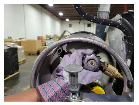
• Once you are sure the connection is secure, turn the shut off valve counterclockwise to open the tank.
