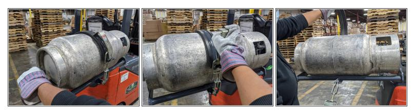
• Release the latch holding the tank to the rack.
