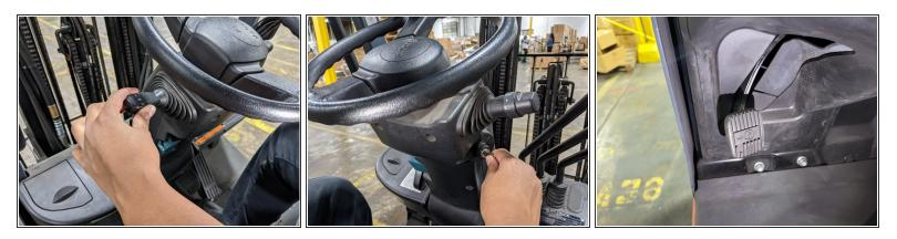
• Put the shifter in neutral, turn the engine off, and engage the emergency brake.
