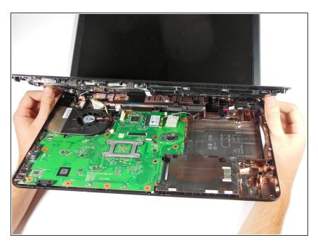
Release all internal latches by working the slack around the motherboard.
