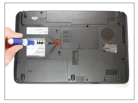
Turn laptop over and remove the 2.5mm "F3" screw using a Phillips #1 screwdriver.
