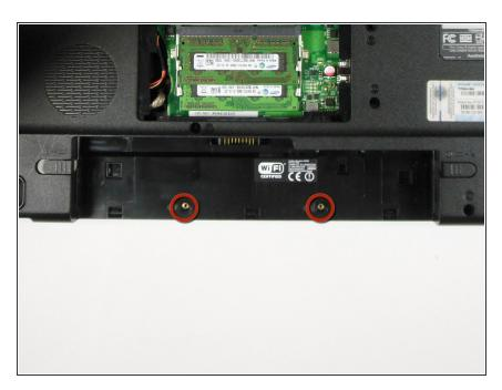
Remove the two 6.0 mm golden (F6) screws shown underneath the battery.
