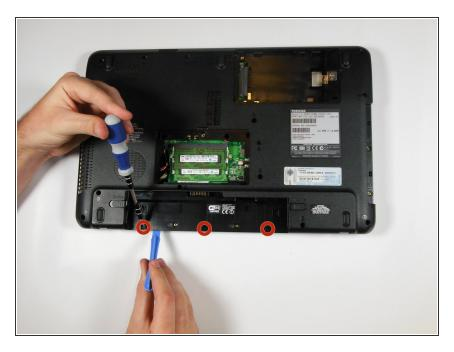
Release the three tabs underneath the battery, using the prying tool.
