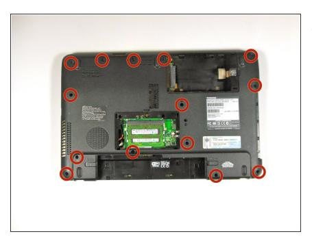
Remove the fourteen 6.0 mm (F6) screws from the back panel using the Phillips #1 screwdriver.
