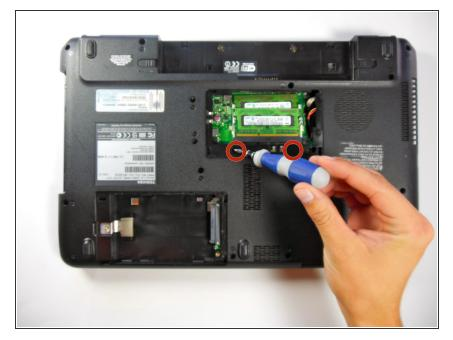
Remove the two 6.0 mm (F6) screws with the Phillips #1 screwdriver.
