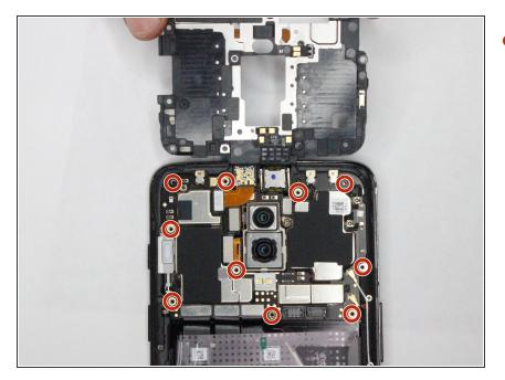
Remove the ten screws holding the motherboard using a Phillips #00 screwdriver.
