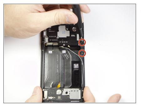
Remove the two 2.3 mm screws using the Phillips #00 screwdriver.
