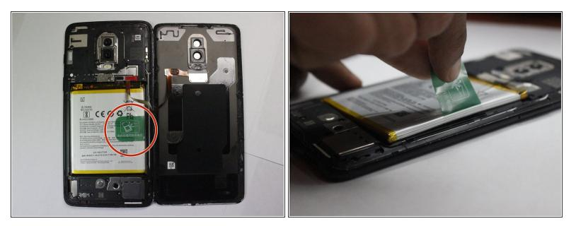
• Grip the green tab connected to the battery and pull the battery directly up and out.
