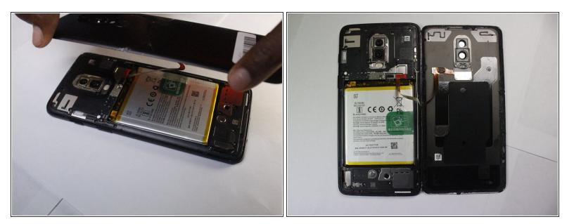
• Gently lift up the back panel, with care not to damage the fingerprint sensor ribbon cable.
