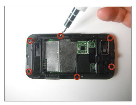
Remove the six 6mm T4 screws with the T4 torque driver.
