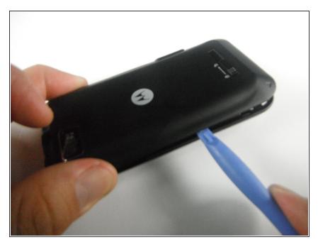
Once wedged in the opening, slide the opening tool around the side of the phone and remove the back cover, setting it aside.
