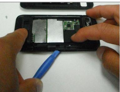
Wedge the plastic opening tool in-between the plastic layer and the front cover.
