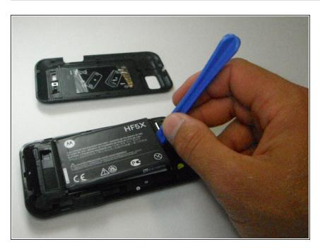
Insert the opening tool between the battery and the battery holder and wedge the battery out.
