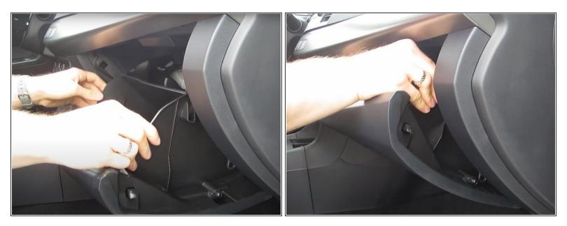
Push both sides of the glove box inwards the same way as in Step 2 and push it back into the housing
