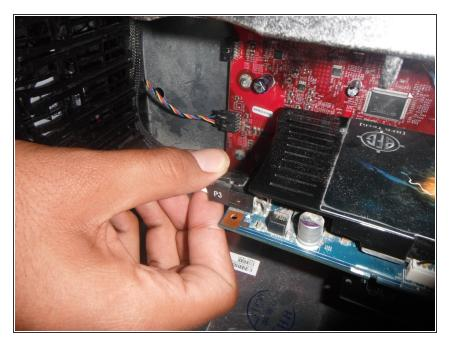
• Unplug the cable labeled "P3" on the left side of the graphics card. Be sure to push the plastic pin all the way down and pull firmly.
