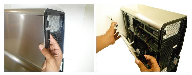
Remove the cover panel on the side of the computer by pulling out the latch on the back panel and pulling the panel downwards towards the ground.
