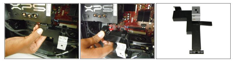
Remove the support underneath the processor cooler by pressing down on the latch at the top of the support and pulling the support towards you.
