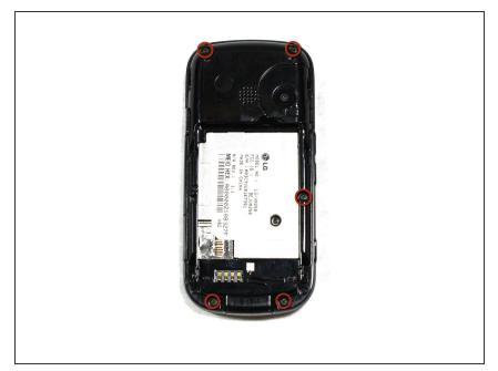
Remove the five 3.0mm Phillips #000 screws along the edge of the rear case.
