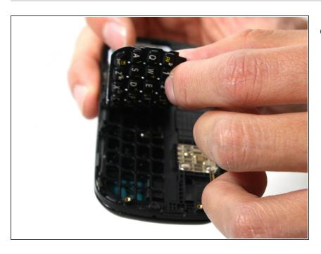
Lift the silicon keypad away from the rest of the phone.
