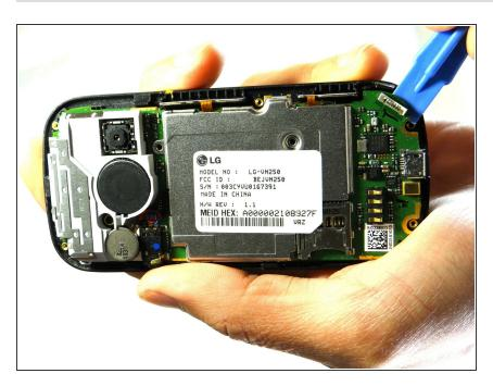
Use the plastic opening tool to pry the motherboard loose.
