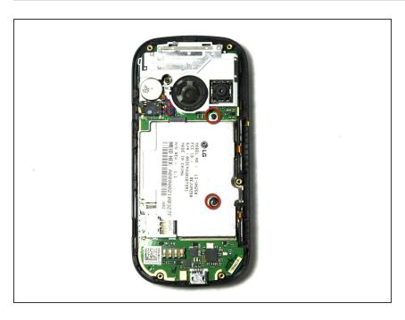
Remove the two 2.9 mm Phillips #000 screws that are slightly offcentered to the right.
