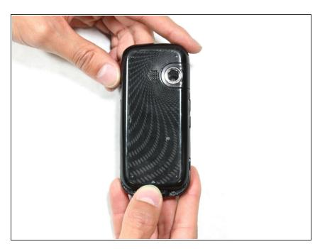
Apply an upward force to slide the back cover off.
