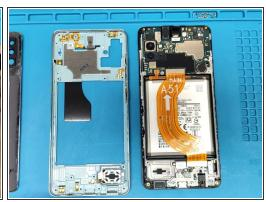
Only use plastic tools to separate the metal frame.
