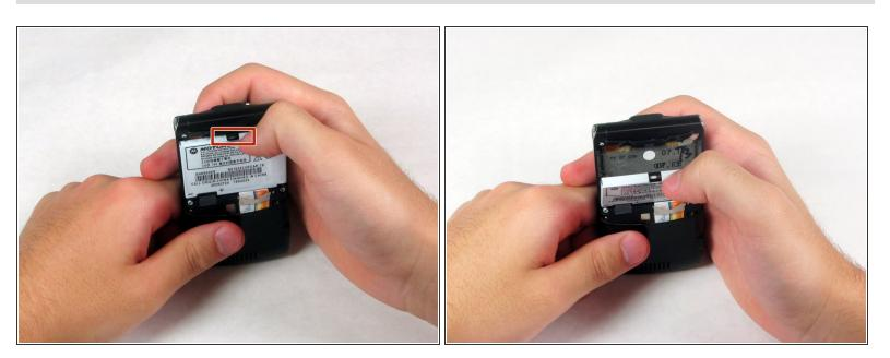
• Remove the battery by pushing down on the top and pulling it away from the phone.
