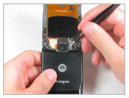
Using a pair of tweezers gently grab and remove the camera from the phone.
