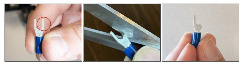
• Cut off the spade terminal's right prong with scissors.
