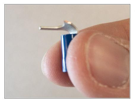
• Bend the spade terminal forward at a 90-degree angle.
