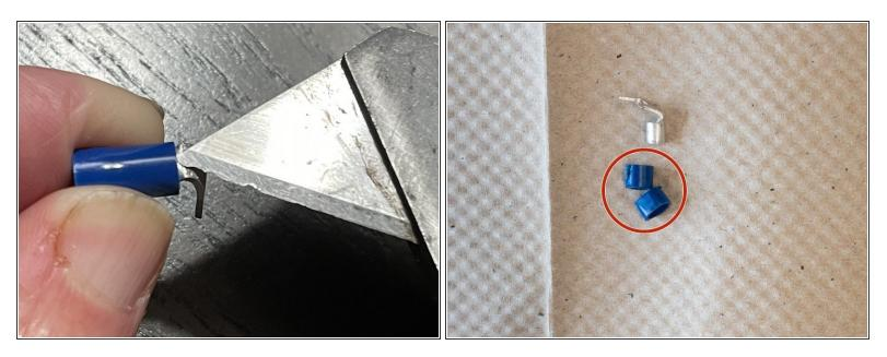
• Slice the blue plastic off of the spade terminal with the boxcutter/Exacto-knife.
