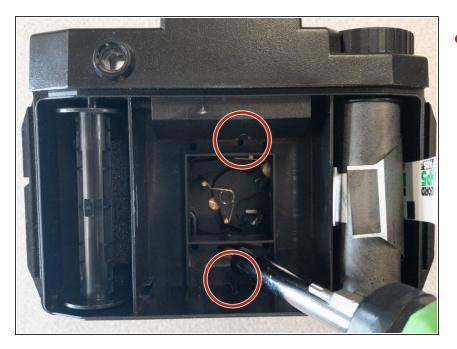
Screw the shutter piece back into place using a Phillips #00 screwdriver.
