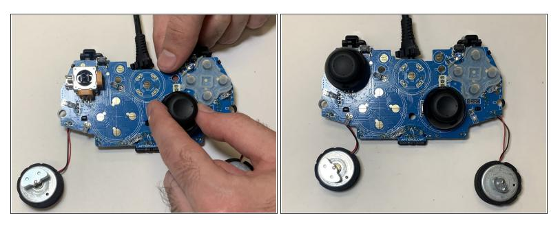
• Place the new joystick into position and press until the joystick makes a click.
