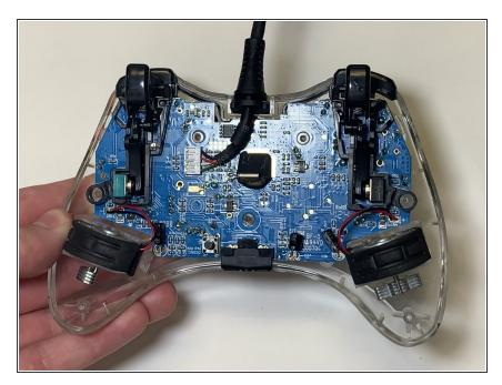
• Remove the back cover from the controller and set it aside.
