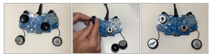
• Wiggle and pull the joystick until it comes off of the circuit board.
