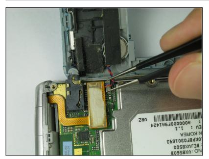
Use tweezers to pull the clear end of the red and blue speaker cables away from motherboard.
