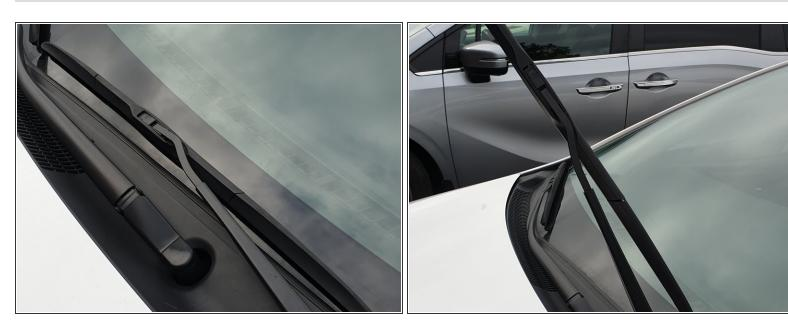
Lift up the windshield wiper you're replacing.
