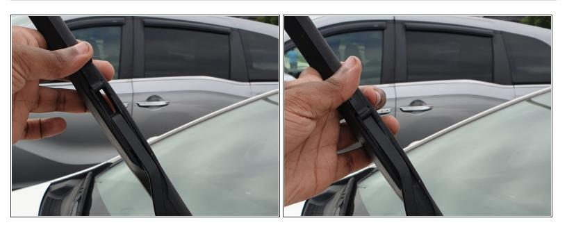
Push the wiper blade downwards until it locks into place.
