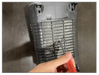
• Use a Phillips #0 screwdriver to remove the 3.5 mm screw holding the bottom case to the device.
