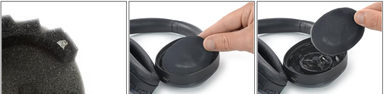
**⚠** The protective cloth in the inside of the ear cups is glued to small foam spacers. These foam spacers are glued to the headphone frame with small pieces of adhesive tape. During the following step make sure to remove the protective cloth including the foam spacers and not to rip the cloth off them.
