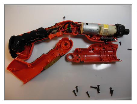
• Lift one side of the drill casing off of the drill. Note that the drill casing consists of two pieces on either side of the drill.
