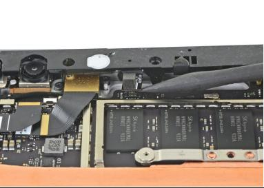
Use the pointed end of a spudger to pry up the connector next to the rear-facing camera and disconnect it.
