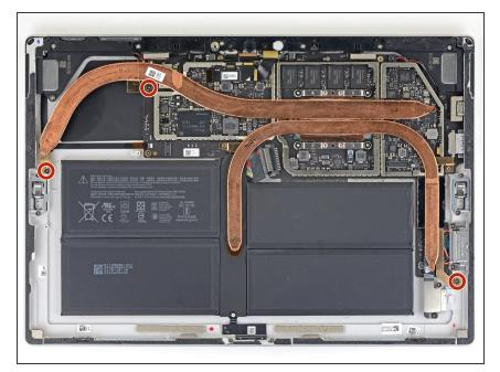
Use a T3 Torx screwdriver to remove the three 2.7 mm screws securing the heatsink.
