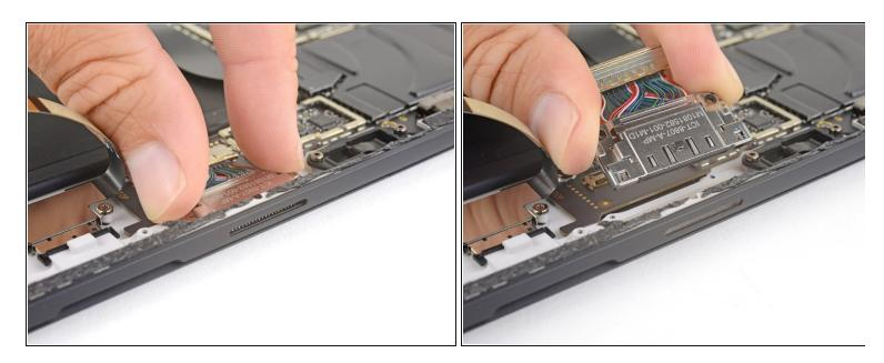
Gently pull the SurfaceConnect port out of its recess in the case and remove it.
