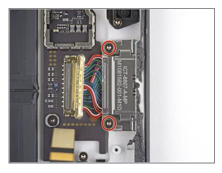
Use a T5 Torx driver to remove the two 3.7 mm screws securing the SurfaceConnect port.
