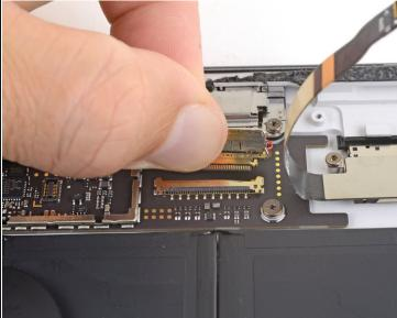
Slide the SurfaceConnect port connector out of its socket on the motherboard.
