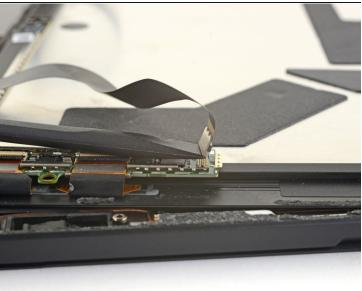
• Use the flat end of a spudger to pry the display interconnect cable straight up and out of its socket on the board.
