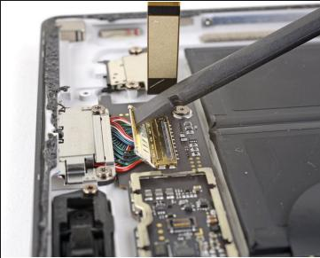
• Use the flat end of a spudger to lift the flap that sits over the SurfaceConnect port connector.
