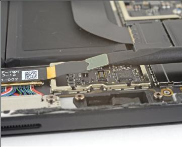
• Use the flat end of a spudger to pry the microSD card reader connector up and out of its socket on the motherboard.
