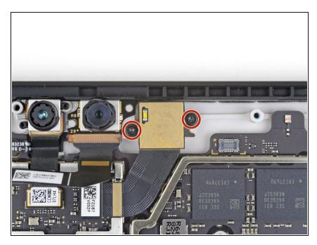
Use a T3 Torx driver to remove the two 2.5 mm screws securing the rear camera.
