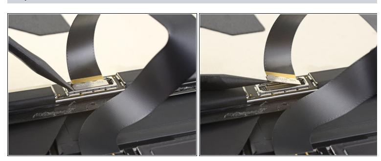
• Use the tip of a spudger to pry the digitizer connector straight up and out of its socket on the screen.
