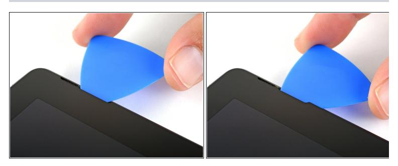
Rotate the pick toward the bottom of the Surface to slide it underneath the lower edge of the speaker cutout.
