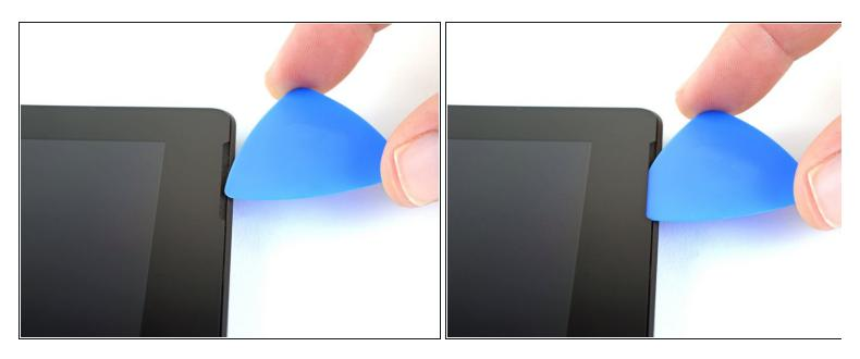
Insert an opening pick into the speaker opening on the screen and slide the pick under the glass. Do not press the pick into the speaker grille, as the grille is easily torn.
