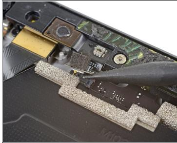
Use the point of a spudger to pry the microphone connector straight up and out of its socket on the motherboard.
