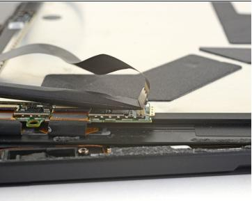
• Use the flat end of a spudger to pry the display interconnect cable straight up and out of its socket on the board.
