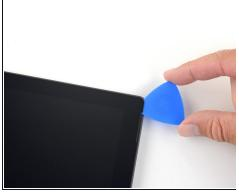
Once you cut the adhesive over the antennas (8.5 inches, or 22 cm, away from the left edge), slide the pick the rest of the way along the top edge of the surface and round the top right corner to slice through any remaining adhesive.
