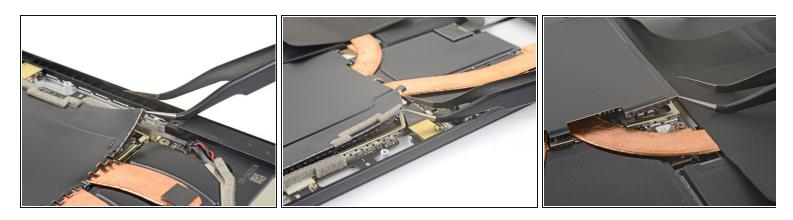
Repeat the last step for each corner of the EMI shield covering the heat sink.
