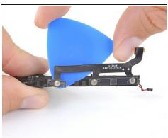
Slide an opening pick under the volume and power buttons to separate the adhesive securing the buttons to the speaker.
