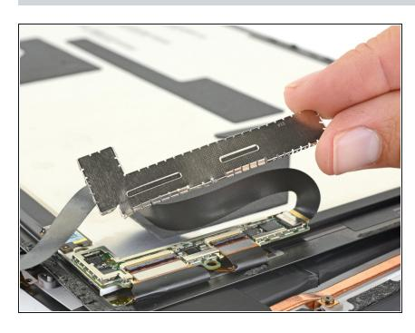
Lift the EMI shield away from the display board and remove it.
