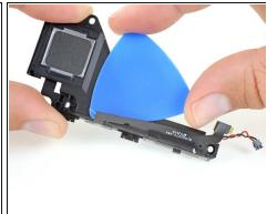
• Slide an opening pick under the volume and power button cable to separate the adhesive securing the cable to the speaker.
