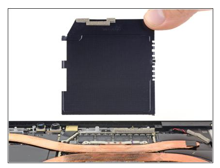
• Remove the heat sink shield.
