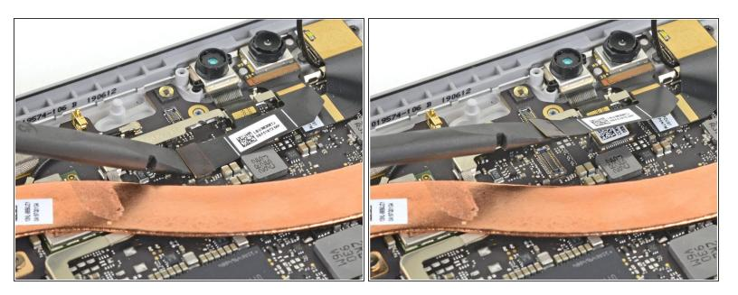
Use the flat end of a spudger to pry up the camera connector and disconnect it from the motherboard.
