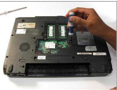
Remove the 4.0 mm screw above the small metal tab with a Phillips 00 screwdriver.
