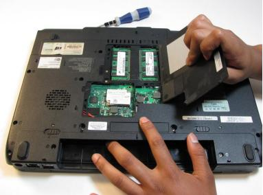
• With your fingers, carefully remove the middle panel by lifting the edge with the indent.
