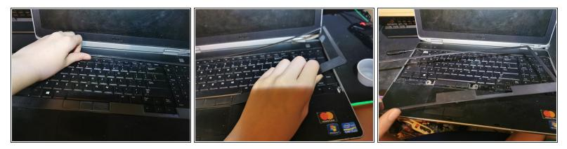
• Use your fingernail or opening tool to remove the keyboard bezel.
