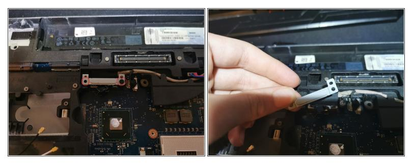
• Unscrew and remove the bracket.
