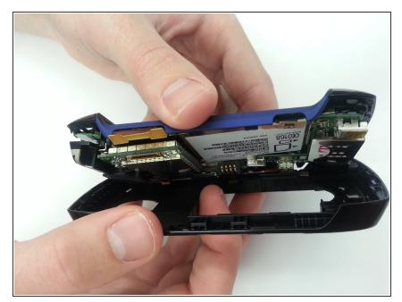
After removal of the back screws, use the Plastic Opening Tool to carefully separate the top and bottom halves of the device.
