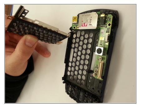
Using the appropriate size Phillips screwdriver, remove any screws that are attached or associated with the keypad and carefully remove keypad from the device.
