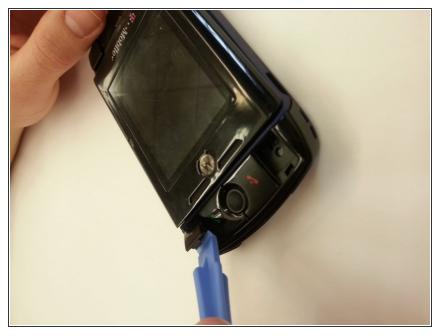
• When looking at the front of the phone, use the Plastic Opening Tool to pry off the four buttons located in each of the corners on the front.
