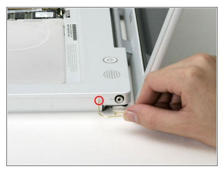
Use a straightened paperclip to open the optical drive tray, and pull it out about halfway.
