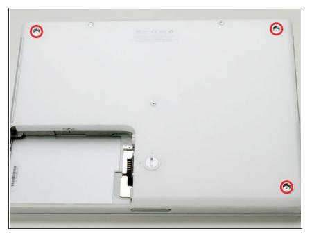
• Remove the three newly-revealed Phillips screws.
