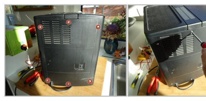
• The rear panel and side panels are attached with six phillips screws #2. Screw them out.
