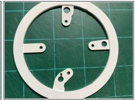
Undo the four screws the remove the white defuser piece (I lost a screw)
