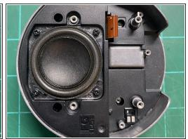
Remember to un latch the ribbon cable before pulling the circuit board up
