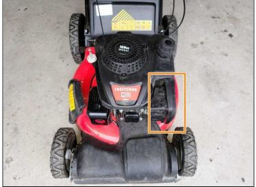
• Remove the black plastic cover to the air filter using a screwdriver to remove the single screw that secures the cover.
