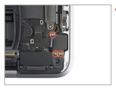
Use a T3 Torx driver to remove the three 4.4 mm screws securing the headphone jack to the case.
